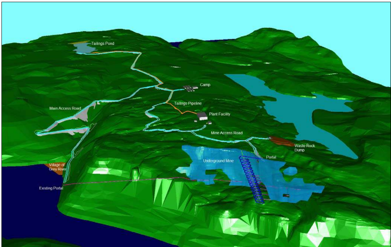
Figure 17.1: Isometric view of the Grey River project site infrastructure and underground mine workings (no scale)
